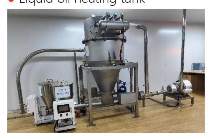
Automatic metering and batching tank
