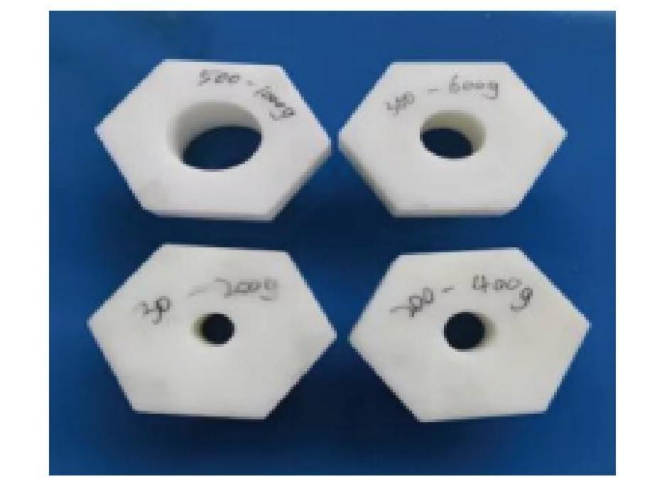
Four types of molds can be replaced, 30g-1500g
